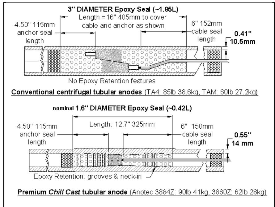
**Figure 6: Epoxy Seal Diameters Compared**
