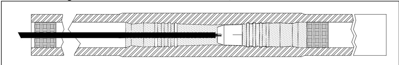
Note the retention grooves and taper seat on the anode ID; proprietary to Chill Cast Tubulars from Anotec
