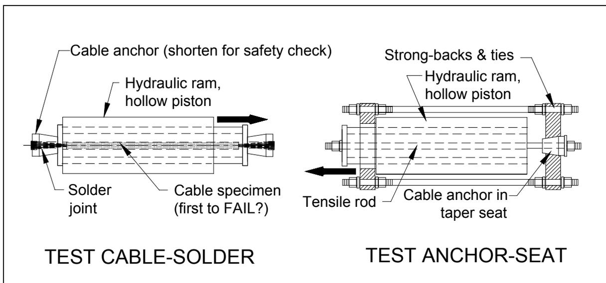
**Figure 5: Cable-Connection Strength Test Apparatus**
