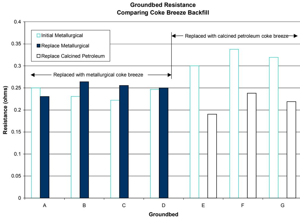
**Figure 7 - Comparison of Deep Anodes Replaced with Different Coke Breeze**
