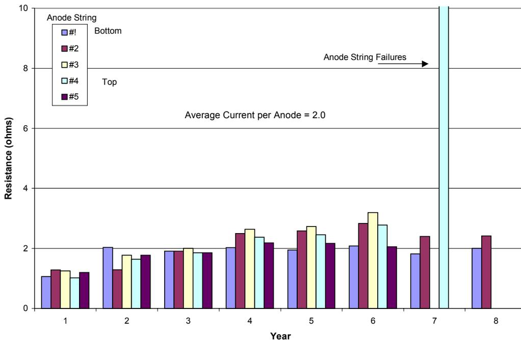
**Figure 16 - Anode String Failures with Time**
