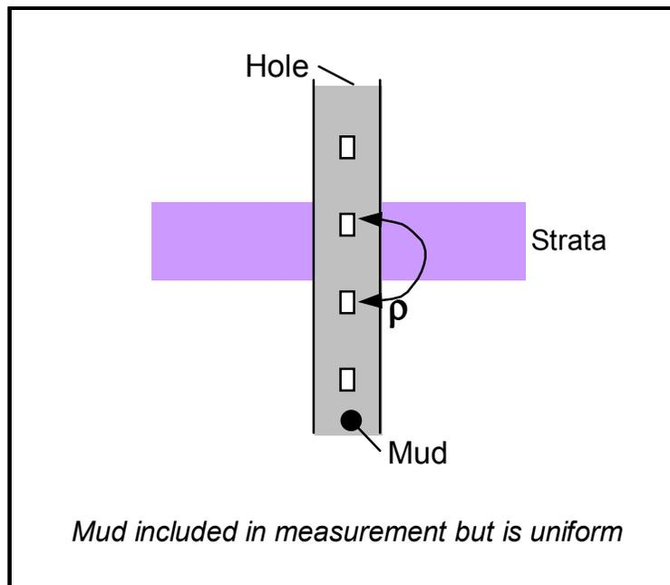
**Figure 12 - Soil Resistivity Log includes Drilling Mud in Reading**
