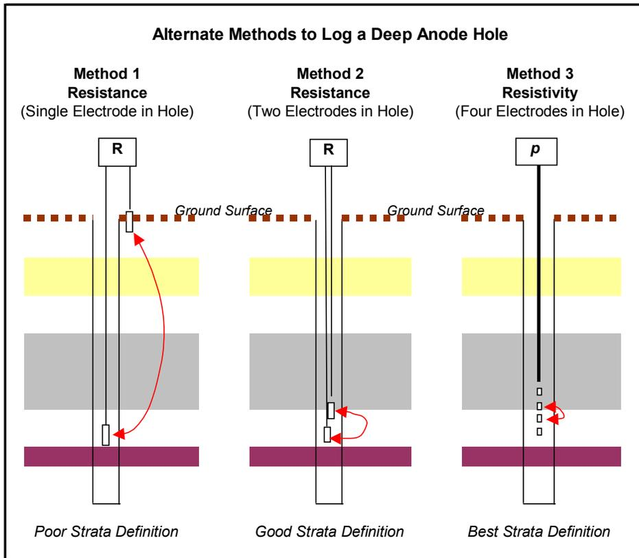
**Figure 11 - Soil Resistivity Logging Methods**
