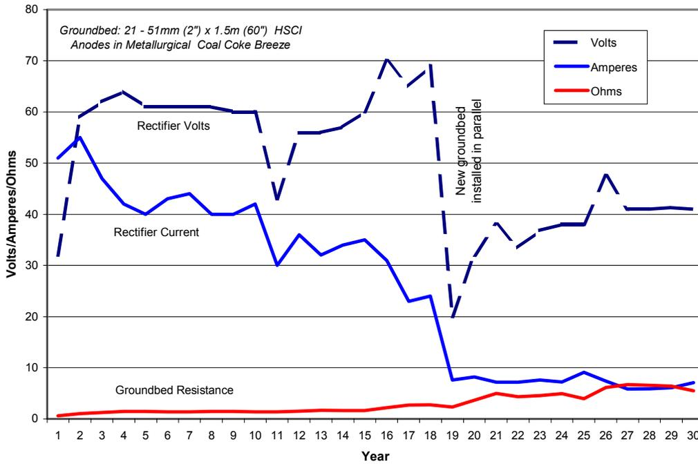
**Figure 13 - History of a Deep Anode Installed in 1964**
