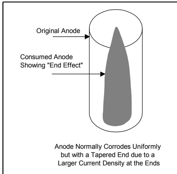
**Figure 3 - Normal Anode Consumption**
