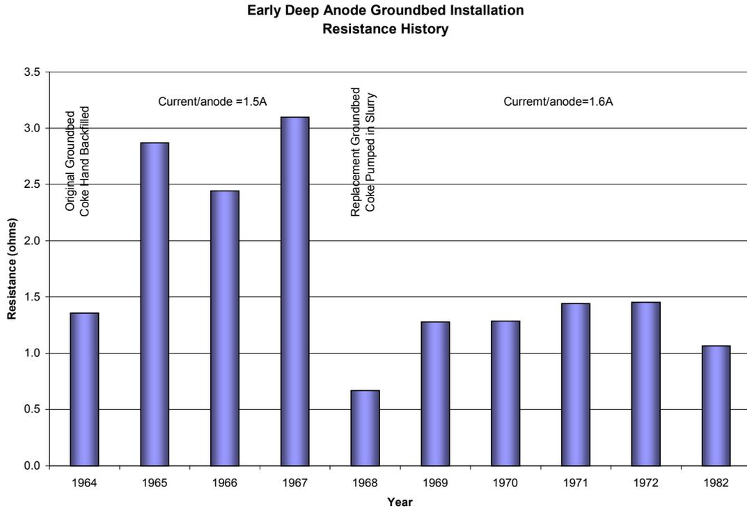
**Figure 1 - Deep Anode Installed in 1964 (Original was hand backfilled while replacement pumped coke in slurry.)**
