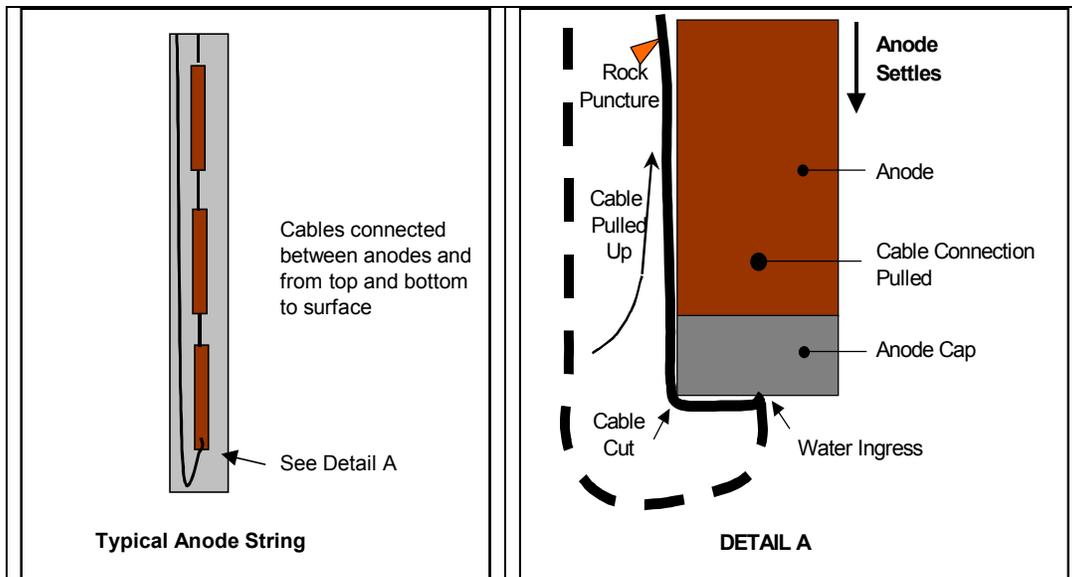
Figure 6 - Typical Anode String in Early Installations Showing Possible Cable Failures
