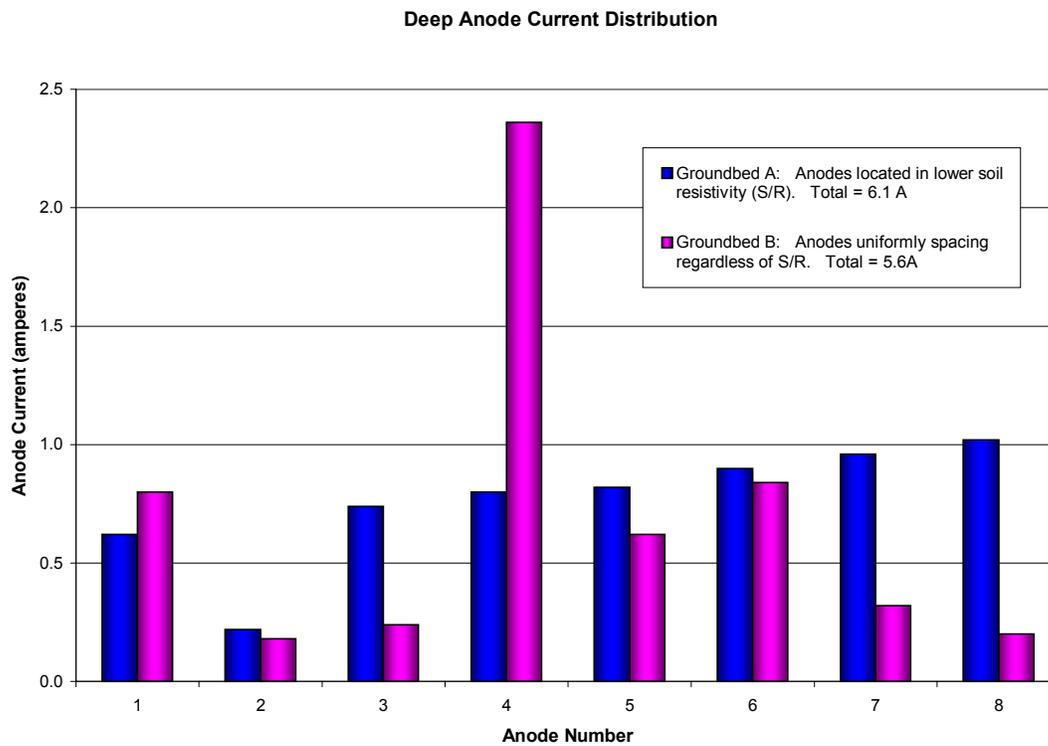
Figure 10 - Anodes Uniformly Spaced Compared to Others Located with Log
