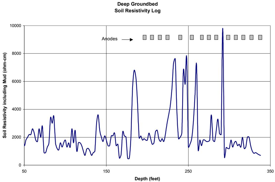
**Figure 8 - Sample Soil Resistivity Log**
