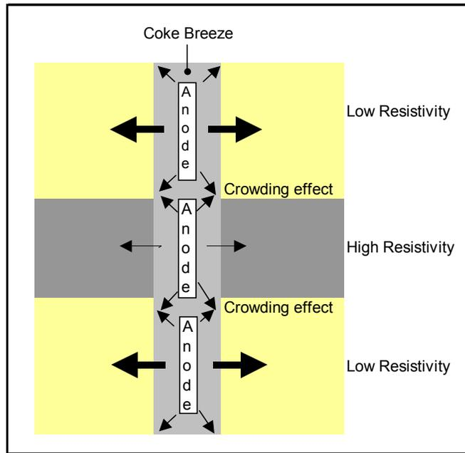
Figure 9 - Illustration of Current Crowding Effect Between Anodes
