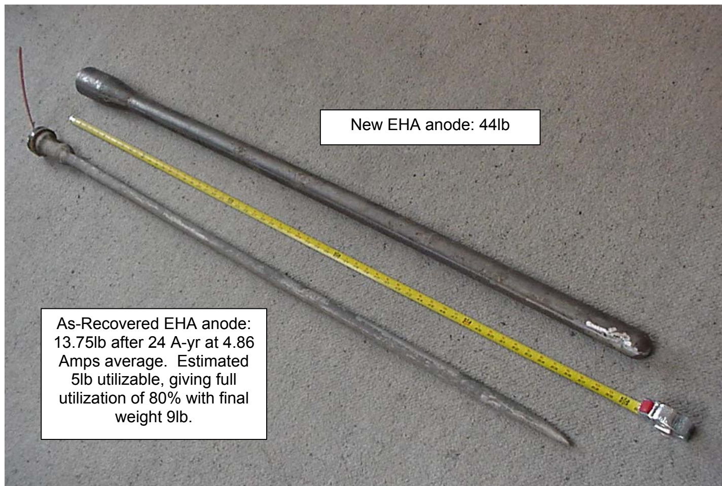
Figure 1: Type EHA 2 x 60" 44lb anodes before and after consumption
